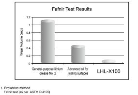
2. Test conditions (ASTM D 4170) Bearings: ANDREWS W 5/8 (Use 2 sets.) Load: 2450 N (Contact pres sure: 1861 MPa) Angle of oscillation: 12 degrees (Average rolling speed: 0.065 m/s) Oscillation cycle: 25 Hz Time: 22 hours Temperature: 25 degrees C Amount of grease per bearing set: 1.0±0.05g Measured amount of wear: Wear of each race way grinder
